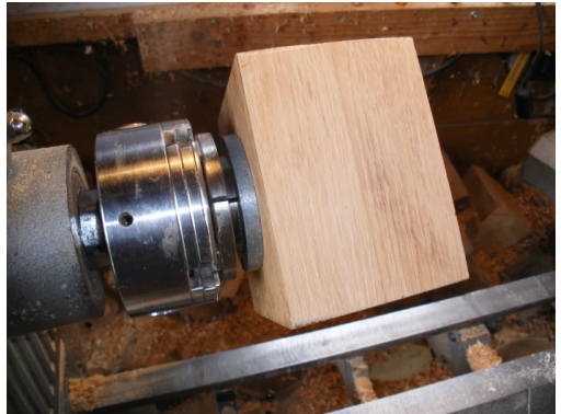
Oak block secured using faceplate ring.
